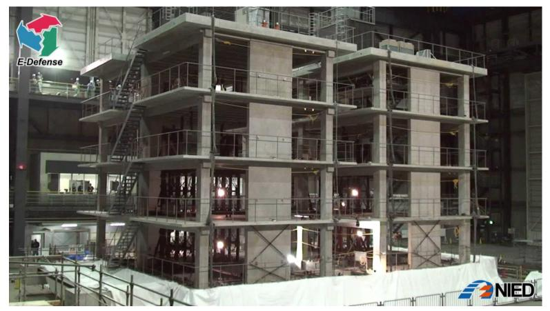
Earthquake simulation to confirm the durability of the building
